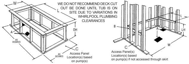
• All dimensions should be taken from tub at jobsite and adjusted as necessary. Always refer to the model specification sheet. Specifications subject to change without notice and installations vary based on model, and whirlpool plumbing systems.
